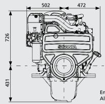
Engine with heat exchanger All dimensions in mm
