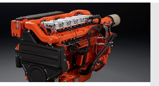
The marine engines from Scania are based on a robust design with a strength optimised cylinder block containing wet cylinder liners that can easily be exchanged. Individual cylinder heads with 4 valves per cylinder promotes repairability and fuel economy. The engines are type approved in all major classification societies.
