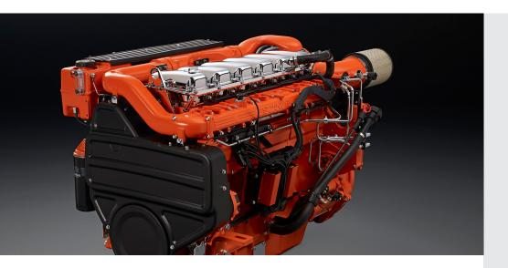
The marine engines from Scania are based on a robust design with a strength optimised cylinder block containing wet cylinder liners that can easily be exchanged. Individual cylinder heads with 4 valves per cylinder promotes repairability and fuel economy. The engines are type approved in all major classification societies.
