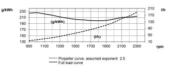
Test conditions Air temperature +25°C. Barometric pressure 100 kPa (750 mmHg). Humidity 30 %. Diesel fuel acc. to ECE R 24 Annex 6. Density of fuel 0.840 kg/dm². Viscosity of fuel 3.0 cSt at 40°C. Energy value 42700 kJ/kg.
